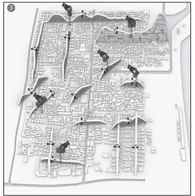
The base shape of the slices is extended by **12m** in width and a grid of **8m\*8m** is formed inside to accommodate the **different functional modules** that will be formed by subsequent stacking.
